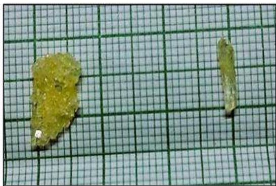
Figure 1 Grown 3 phenyl 2-bromophenol (3P2BP) Crystal
