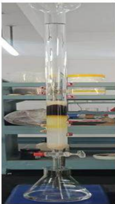
Figure - 3: Column Chromatographic separation
